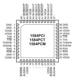
48 Pin Plastic 7mm x 7mm Chip-Scale Package (QFN)
